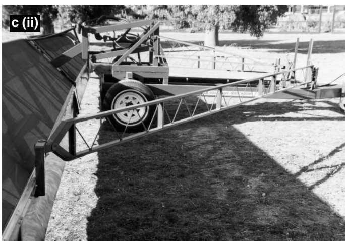
Figure 8c. Bluff plate sprayer – 25 m bluff plate sprayer: commercial model (i) folded position, (ii) towing and hitching layout.
