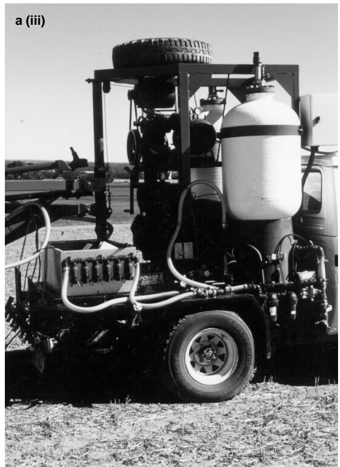
Figure 8a. Bluff plate sprayer – 12 m prototype commercial sprayer: (i) front view in spraying position, (ii) rear view in spraying position, (iii) side view of bluff plate hitch pole and liquid distribution system based on compressed air, mounted on the spray vehicle.
