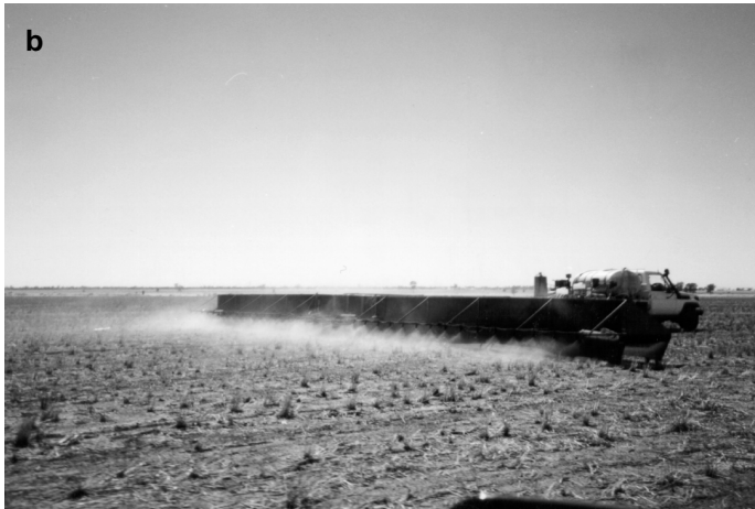
Figure 8b. Bluff plate sprayer – 18 m bluff plate sprayer at Livingston Farm, Moree, New South Wales – sprayer in operation at 25 km h -1 .
