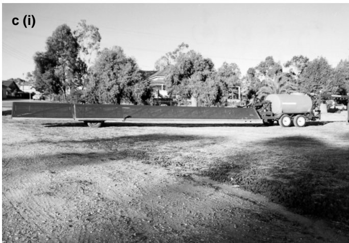
Figure 8b. Bluff plate sprayer – 18 m bluff plate sprayer at Livingston Farm, Moree, New South Wales – sprayer in operation at 25 km h -1 .
